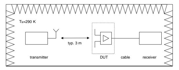
The transmitting antenna is aligned towards the antenna under test (height, polarization).
